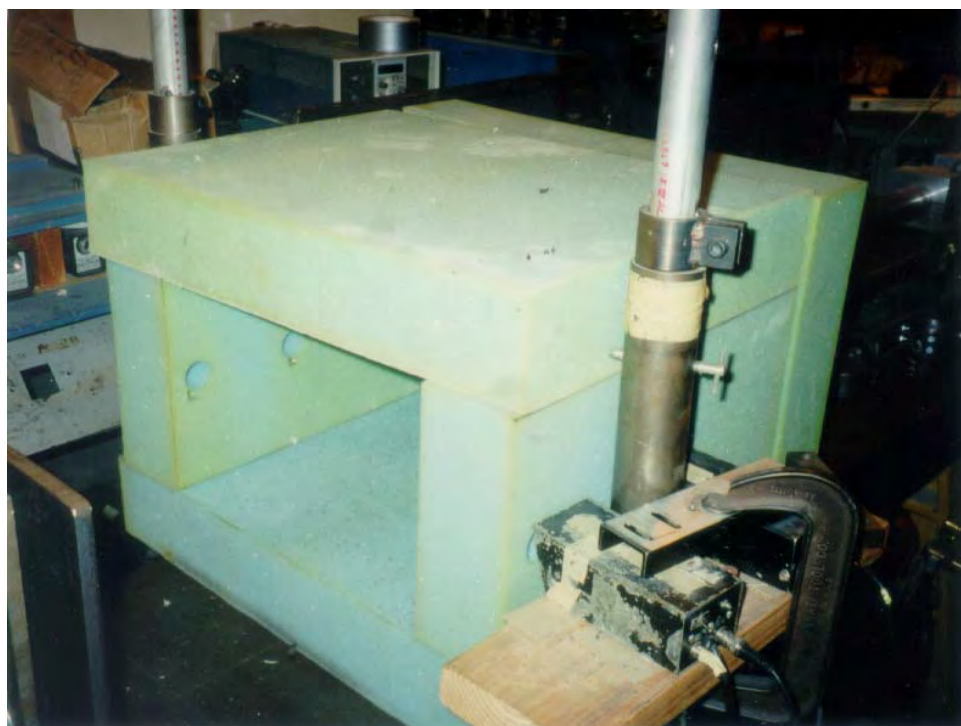
Figure 4. Rebound catcher box.
