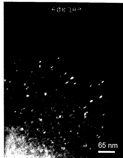
Figure 8. TEM dark field image for the partially devitrified \text{Al}_{85}\text{Ni}_{10}\text{La}_5 amorphous alloy annealed at 245°C for 30 min.
