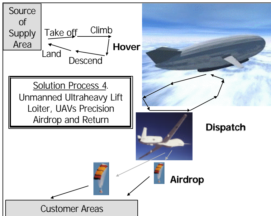
Figure 5. Solution Process 4. Heavy Lift Ship Takes Off and Hovers/Smaller UAVs Airdrop and Return
