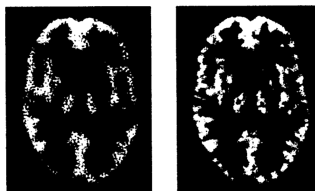
Fig. 14. The same slice of the Hoffman brain phantom shown in Fig. 13 when reconstructed with the 3-D RP algorithm using the Hann window and a cutoff frequency of (left) 0.4 and (right) 0.8 of Nyquist frequency.
