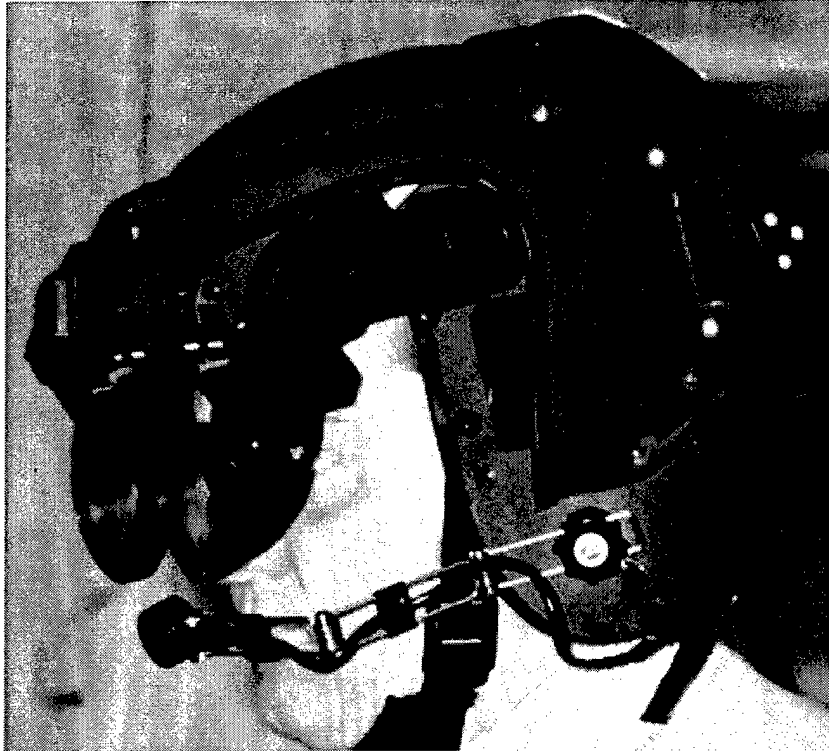
Figure 2. Flight helmet with 53-degree FOV HMD.
