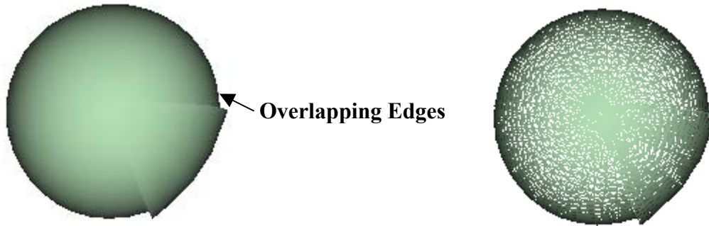
Figure 7.32 Incorrect NURBS Surface Closure.
