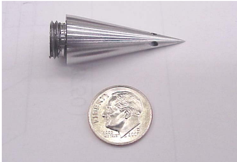
Figure 18. Side view of ramjet cone with fuel injection ports at front.
