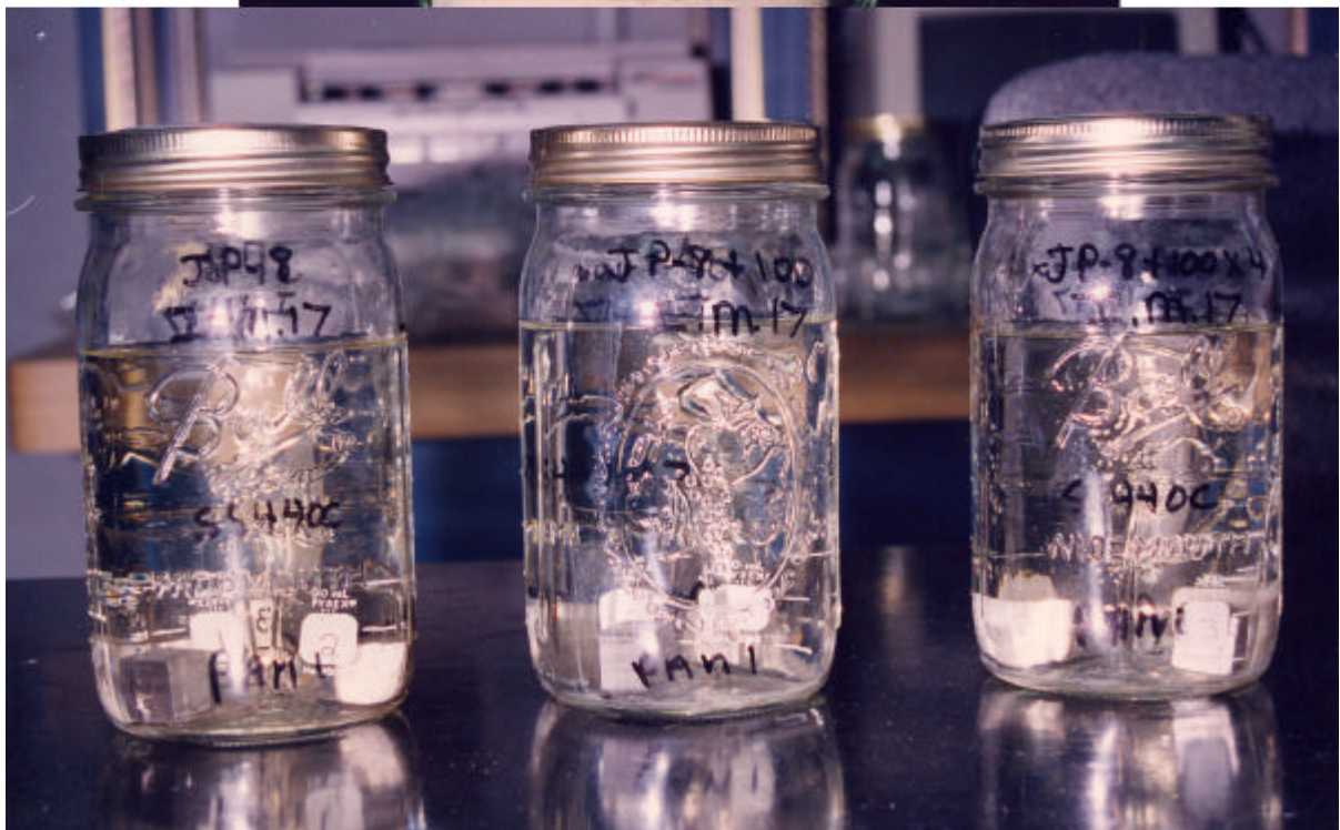
Figure 2: Typical Material / Fuel Test Configuration
