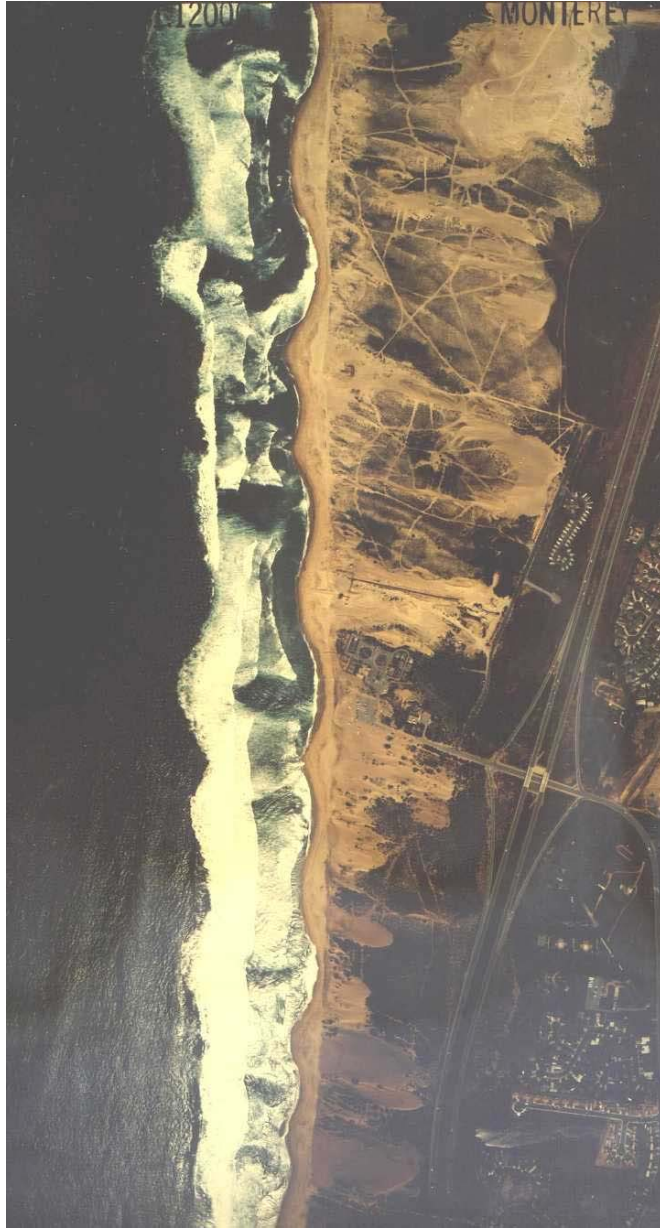
Figure 4. Aerial photo of Southern Monterey Bay taken at low tide on April 1984 with energetic wave conditions showing large beach cusps associated with rip current cells. The cusps and rips are both of O(100-400\text{m}) (Thornton et al. 2003).
