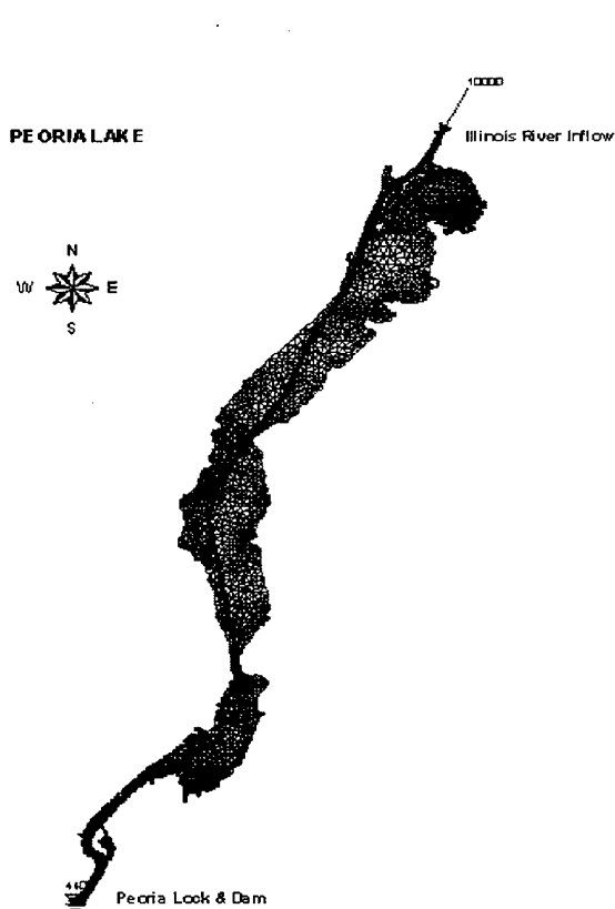
Figure 7. Peoria Lake Pilot Study RMA2/SED2D mesh.
