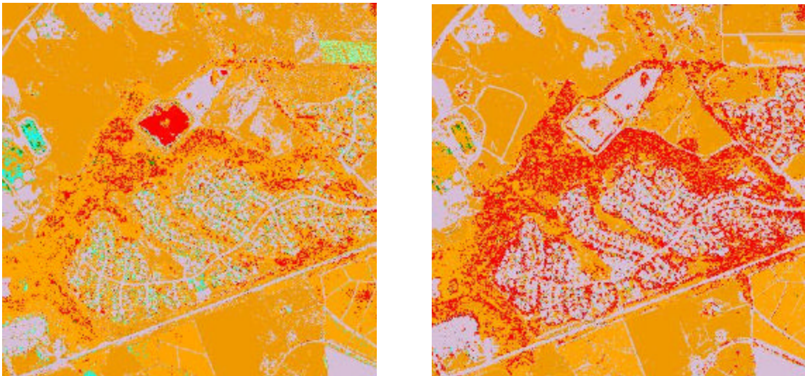
Figure 55. 4 band MSI and 12 band (MSI and texture combined) images of a small residential sub-division displaying greater woodland delineation.
