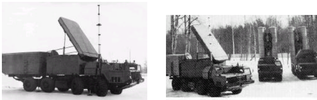
Figure 16. Russian SA-10 associated "Flap Lid" target acquisition radar Right: "Flap Lid" with associated SA-10 "Grumble" missile launchers. (from Jane's Database)
