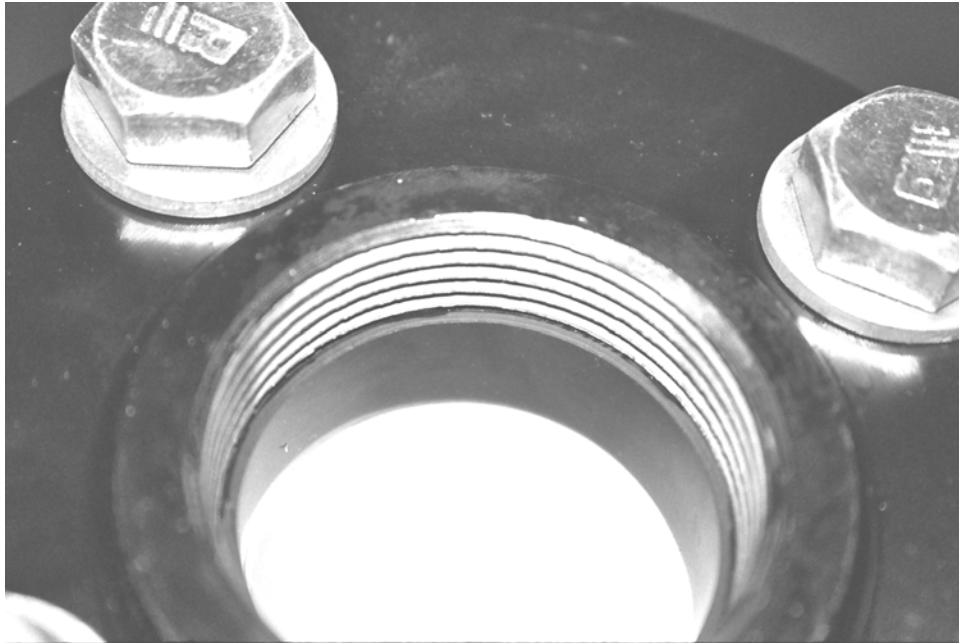
Figure 10. Treaded flanges for mass flow meter
