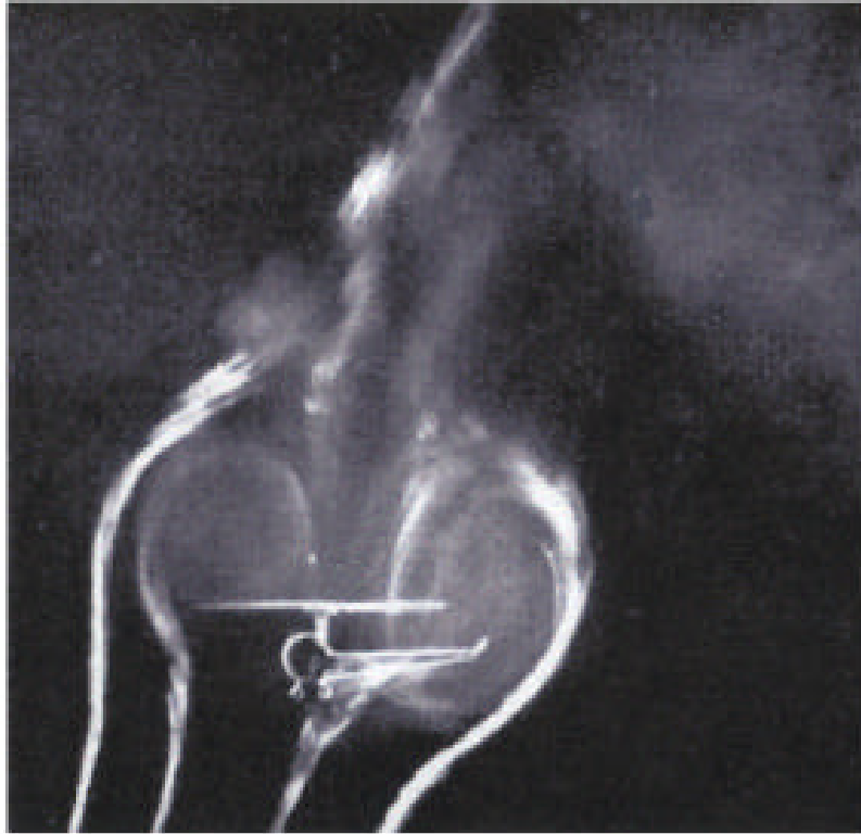
Figure 2. Recirculation During Flight in the VRS. [From: Drees and Hendl Film, 1951]
