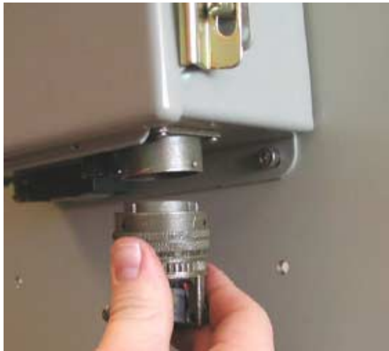
Figure 10. Connecting the Sensor to the NCAP. [From Ref. 4.]
