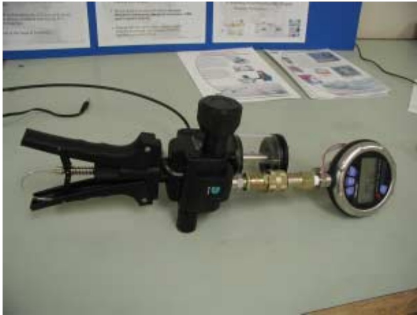
Figure 13. The Crystal XP 2 Digital Test Gauge and Handheld Pump with Bluetooth Adaptor Installed on the Back of the PPC.
