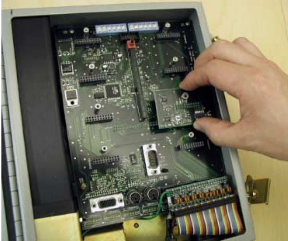
Figure 6. NCAP Interior. This shows an ICP daughter board being installed. [From Ref. 4.]
