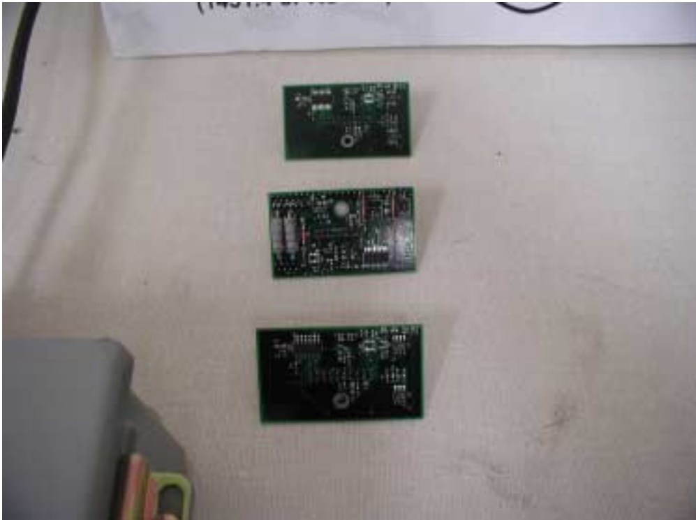
Figure 5. ICP Daughter Boards Used in the NCAP. Top and bottom boards are for a 0 to 5 volt pressure sensor. The middle is for a 4 to 20 mA pressure sensor.
