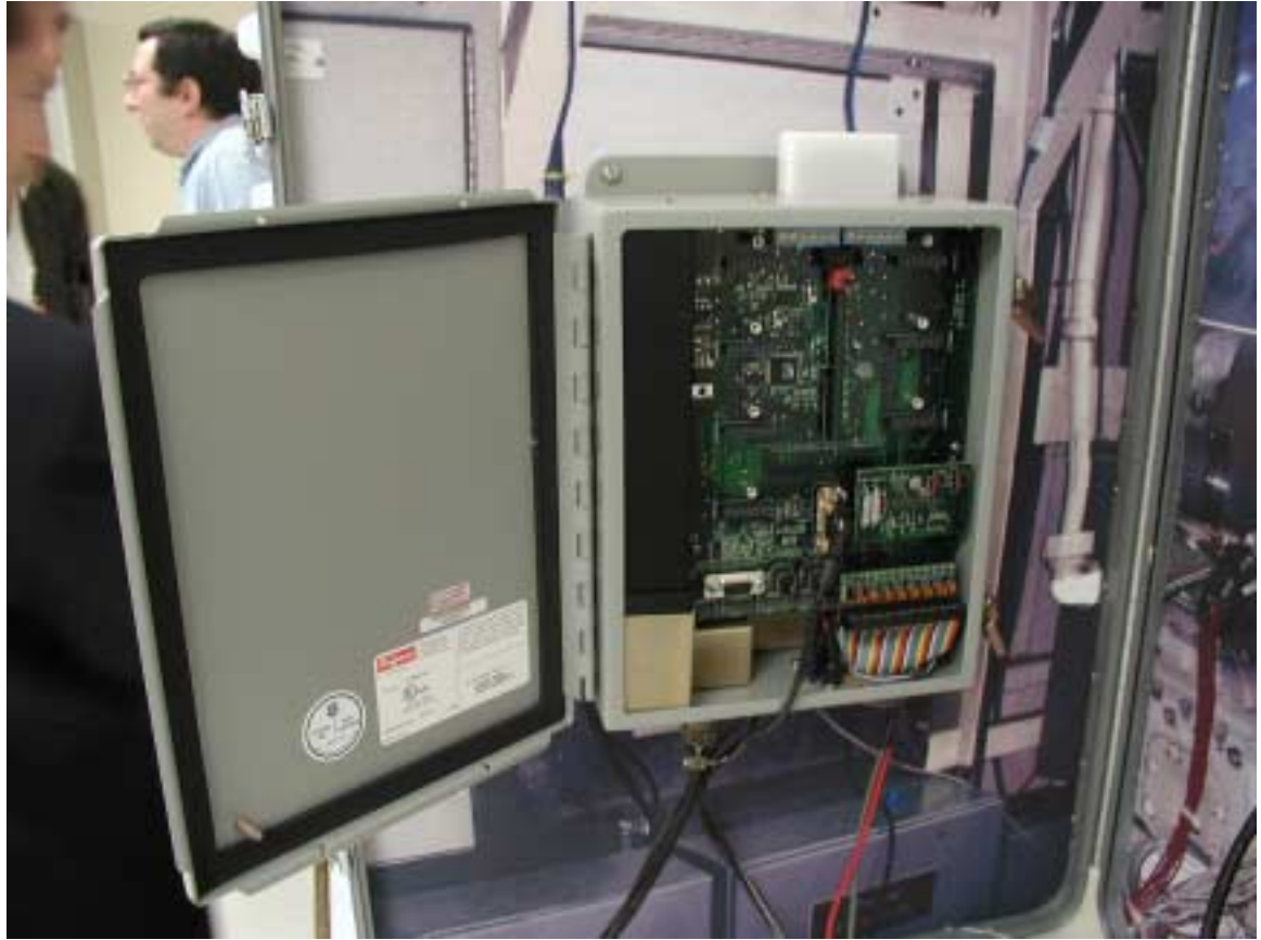
Figure 7. The Interior of the NCAP. The serial port, keyboard, monitor, and mouse inputs can be seen near the bottom of the case.
