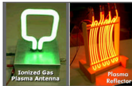
Figure 4: Examples of a plasma loop and reflector antenna using tubes [From 7].
