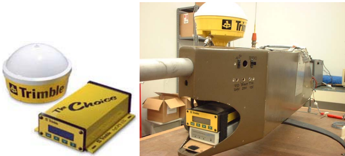
Figure II.4 DGPS Trimble Ag132 Main Components and Mounting Locations.
