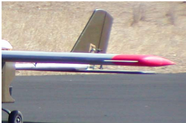
Figure II.9 Pitot-Static Probe Mounted on FROG
