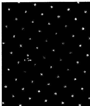
Figure 3.5. Confocal image showing the 1.3 \mu\text{m} patterns attained using the polymer lift-off method.
