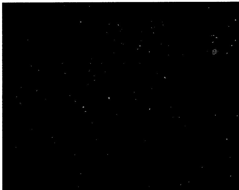
Figure 2.8. Optical micrograph of 40 nm fluorescent spheres bound to an avidin-biotin patterned antibody layer.
