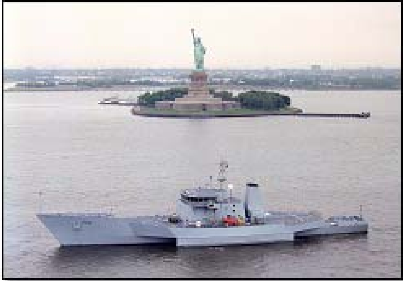
Figure 7-4: RV Triton, Trimaran Hull Technology Demonstrator
