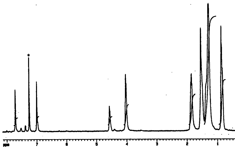
Figure 7. 1 H NMR spectrum of 13b in CDCl 3 . The starred signals at 7.25 ppm is attributed to CHCl 3 solvent.
