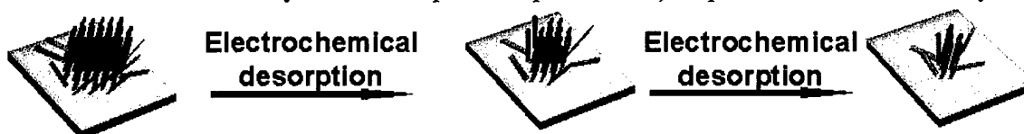
Scheme 8. Alkanethiol patterns are whittled away from the edges using the defect sites at the perimeter.
