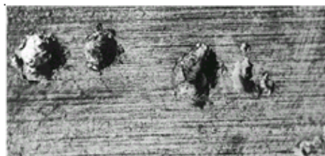
Figure 25. Fusion Craters in a Bearing Race from Scanning Electron Microscope Image. [From Ref. 20].
