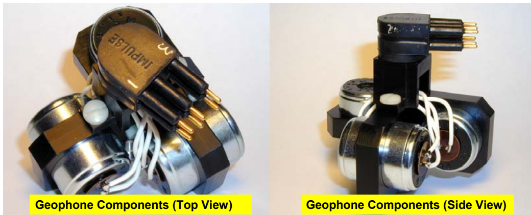
Figure 9. SM-11 Geophones mounted in X-Y-Z coordinates
