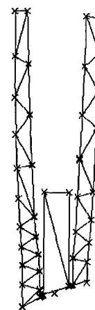
Figure 7.5: Triangles to be bonded on the Graphite-Epoxy 'Blank'
