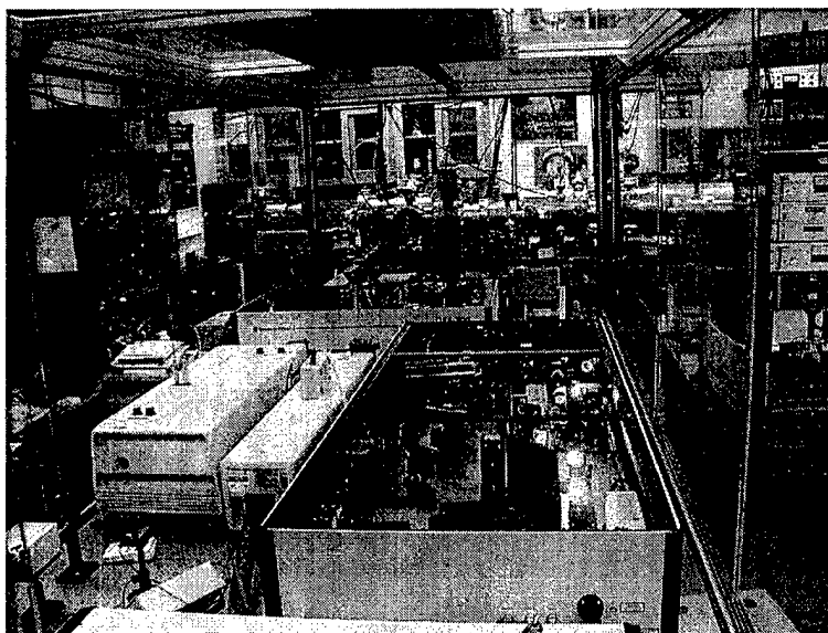
Figure 2. Ti:sapphire femtosecond laser system purchased through DURIP grant.
