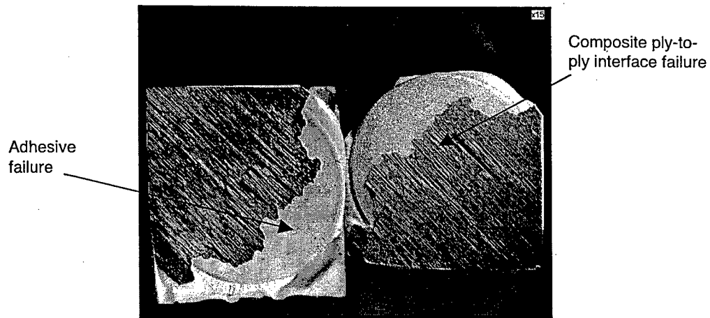
Figure 10. Fracture surface of sample 1, 2, 3, and 4 all appeared to fail within the composite.
