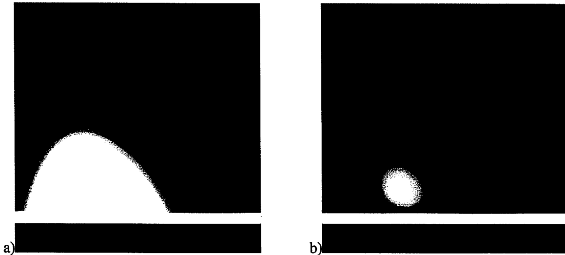
Figure 54: Single band atmospheric attenuation. a) CBZODY6 including refraction and twilight sky radiance from MODTRAN b) CBZODY6 refraction, twilight sky radiance, and attenuation (twilight sky radiance and attenuation from MODTRAN). Indications are that the atmospheric attenuation observed is much less than that predicted by MODTRAN.
