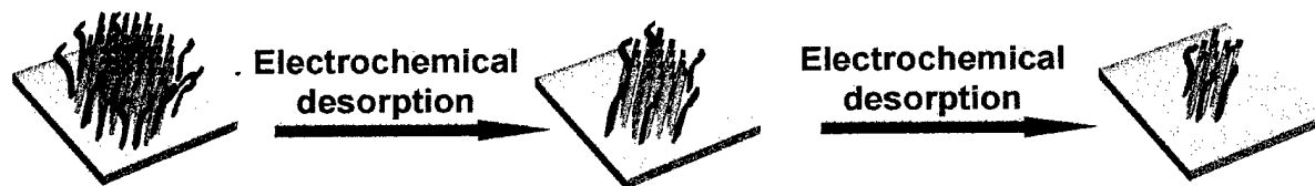
Figure 4. Alkanethiol patterns are whittled away from the edges using the defect sites at the perimeter.
