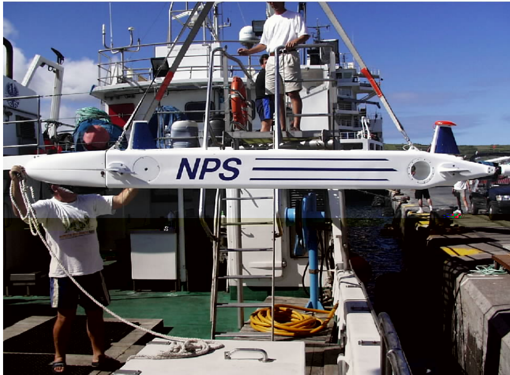
Figure 2. Shipboard handling of NPS' Acoustic Radio Interactive Exploratory Server (ARIES) AUV aboard the Portuguese research vessel ARGUIPELIGO during Azores operations in August 2001 (from NPS Center for AUV Research, 2003b).
