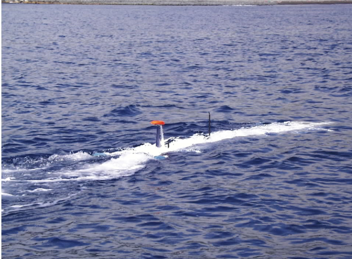
Figure 8. NPS' Acoustic Radio Interactive Exploratory Server (ARIES) AUV performing a GPS pop-up during Azores operations in August 2001 (from Nguyen 2002).
