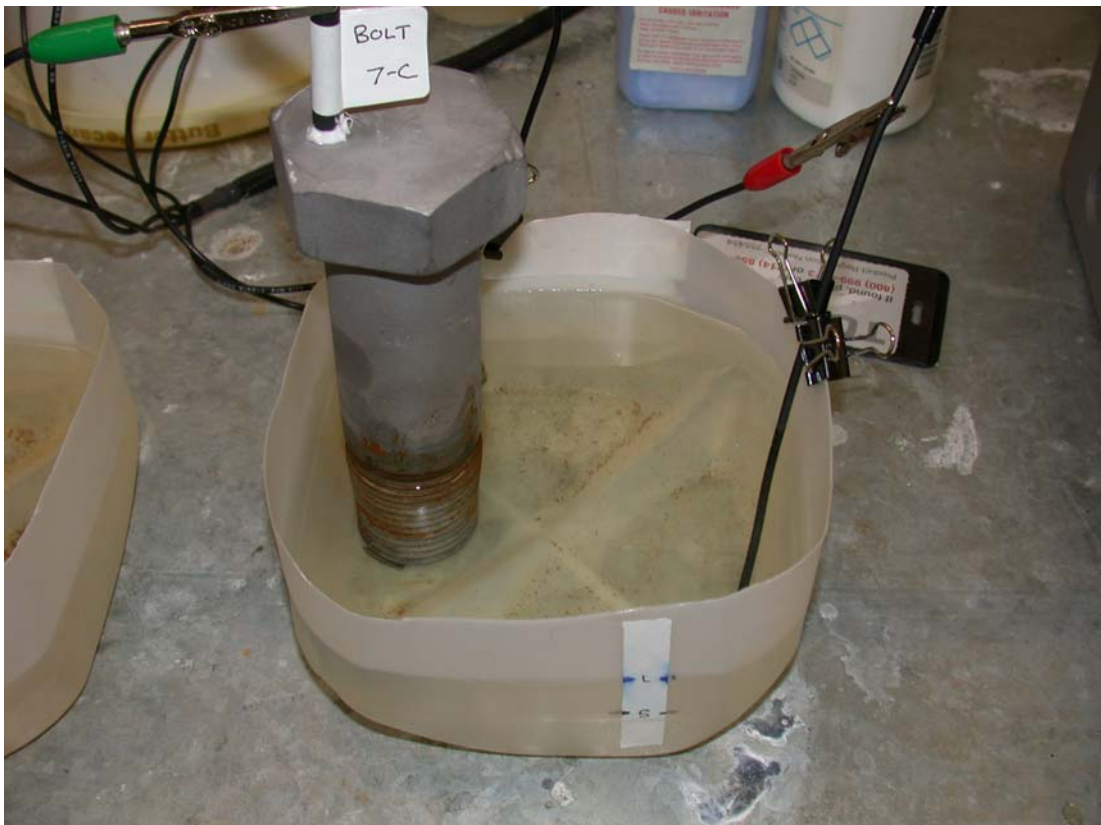
Figure 14. A bolt being tested in Ohio River water.
