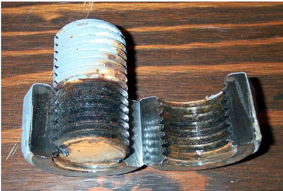
Figure 3. The bolt after the nut was removed.
