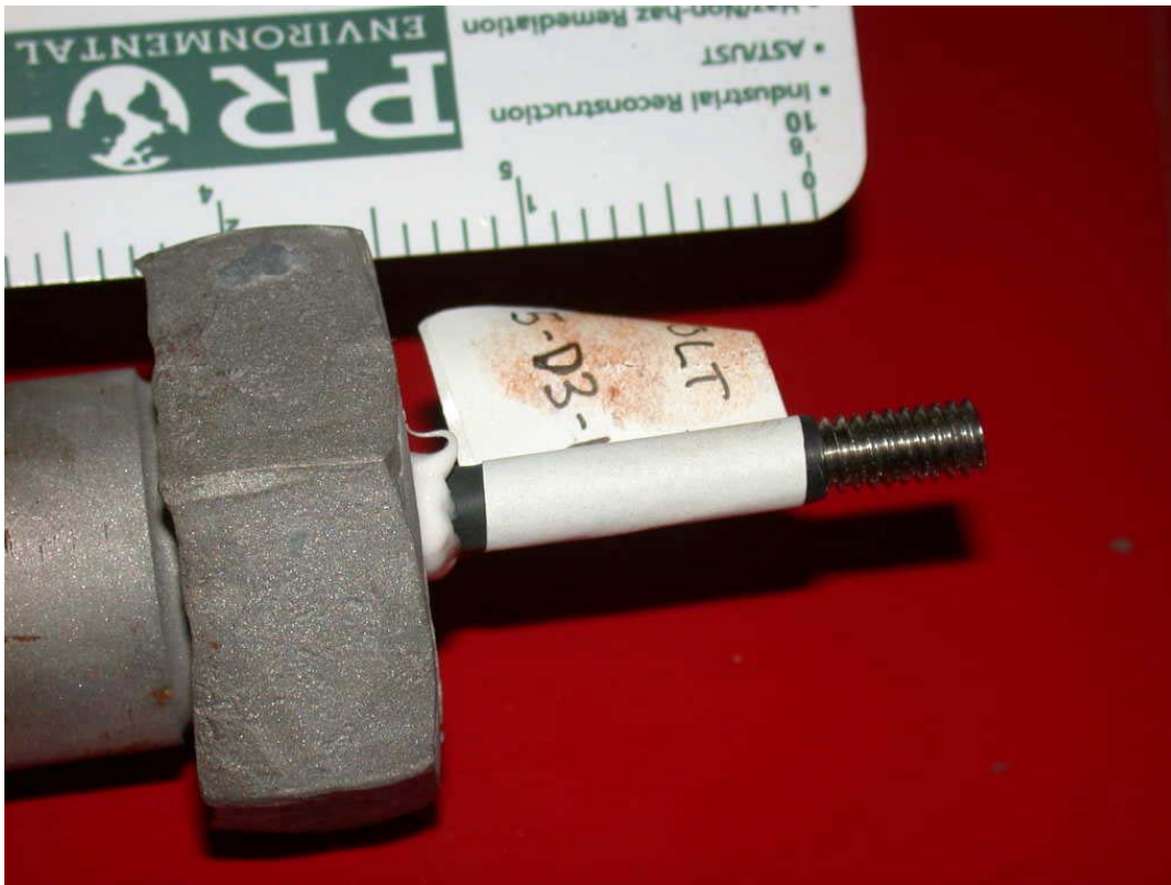
Figure 11. A Type 410 stainless steel bolt ready for testing.
