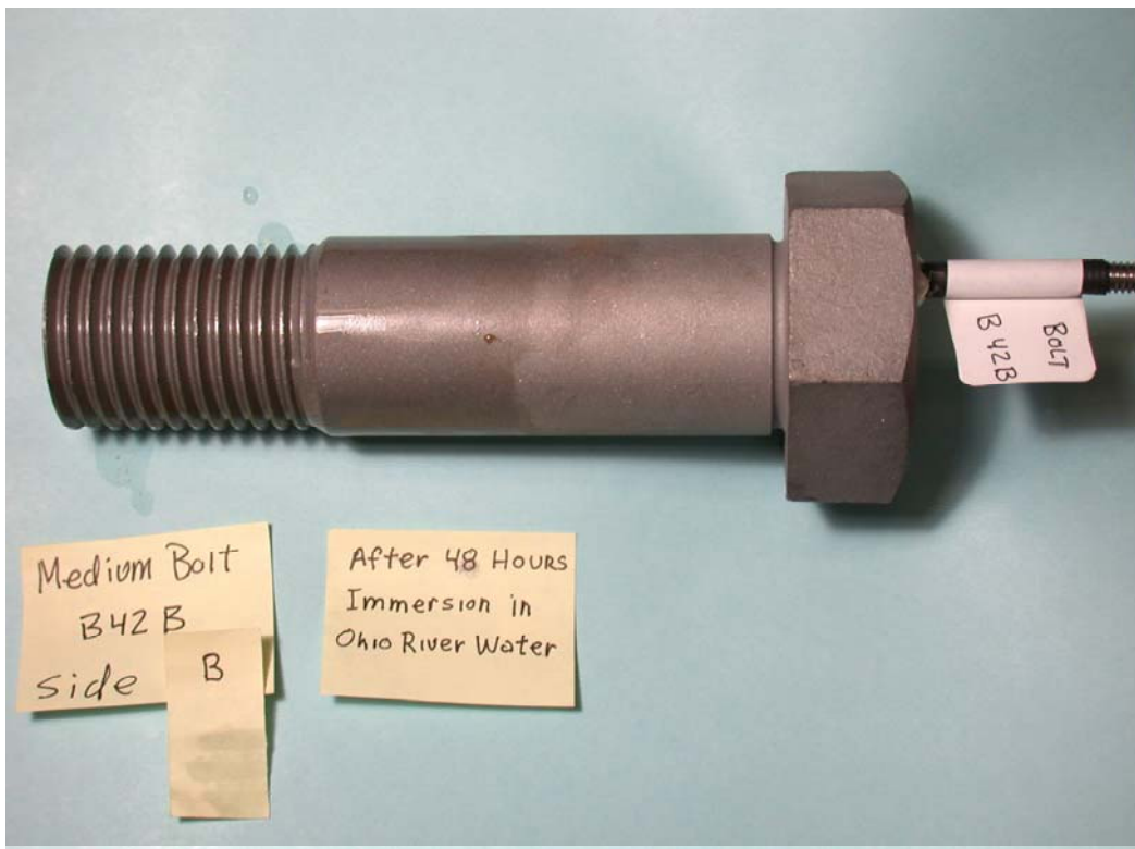
Figure 17. A non-temper embrittled bolt after 48 hours in Ohio River water.
