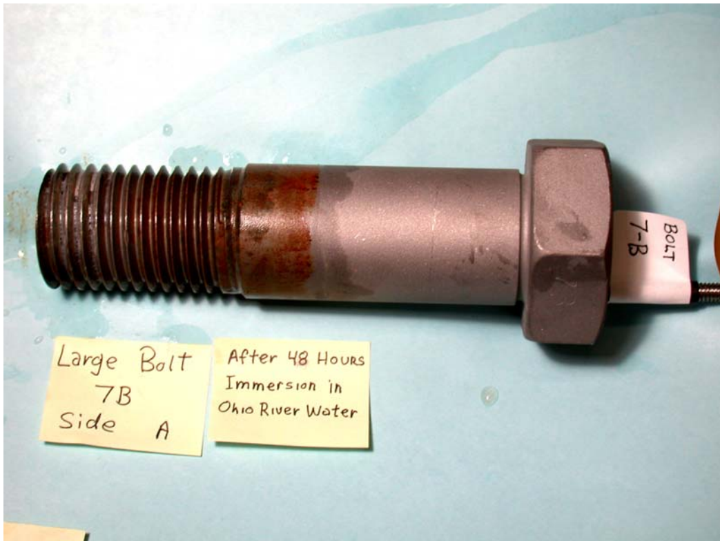
Figure 16. The corrosion products on a temper embrittled bolt after 48 hours immersion in Ohio River water.
