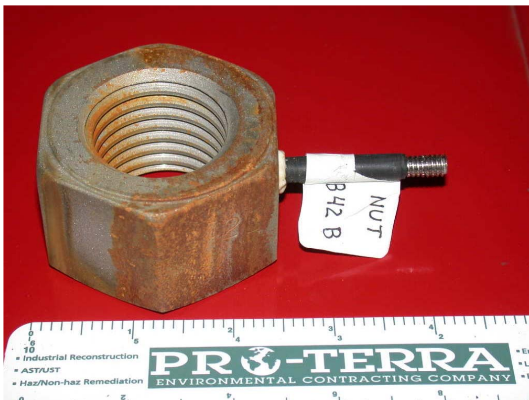
Figure 10. The Nitronic 60 stainless steel nut ready for testing.
