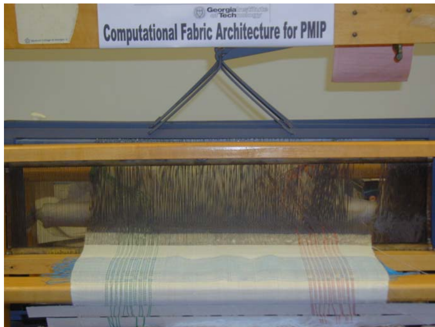
Figure 2. Loom for the Realization of Computational Fabric for PMIP
