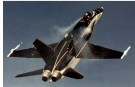
Fig 20 Impact of burst vortices on F-18 fins
