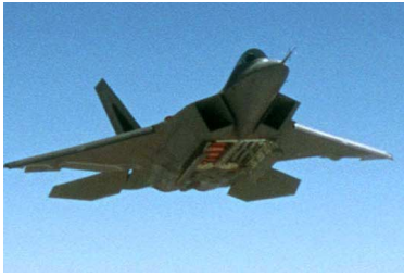
Fig 15 Fuselage chine on F-22
