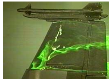
Fig 21 Vortex flow generated by F-18 flap failure
