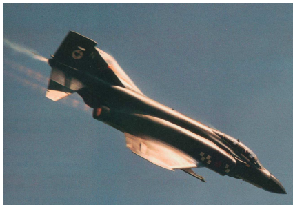
Fig 16 Vortex from intake diverter on F-4
