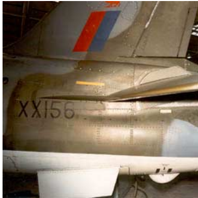
Fig 7 Auxiliary tail surface on Hawk
