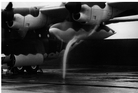
Fig 17 Ground vortex generated by C-130
