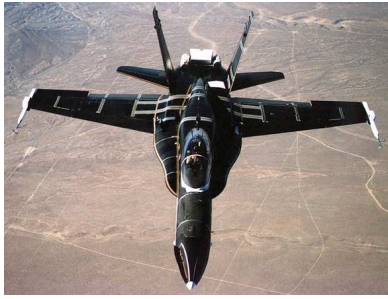
Fig 6 Mechanical strakes on F-18 nose
