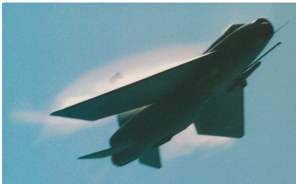
Fig 3 Vortex flow over 60° sweep wing of Lightning
