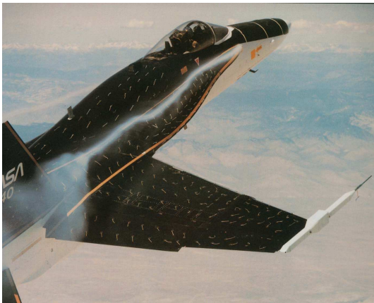
Fig 2 Disorderly flow separation on the upper wing surface of F-18
