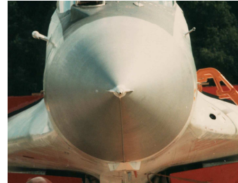
Fig 11 Nose strakes on Mig-29
