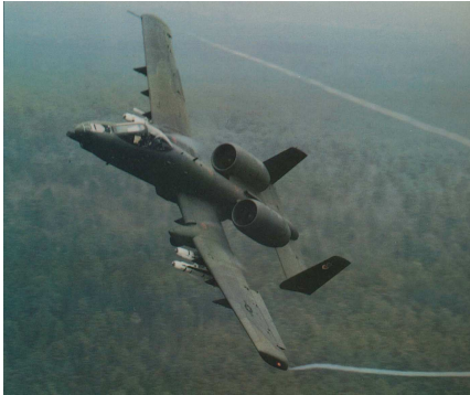
Fig 1 Tip vortices on wings having low sweep: A10 and Tornado
