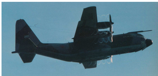
Fig 18 Vortices from C-130 propellers
