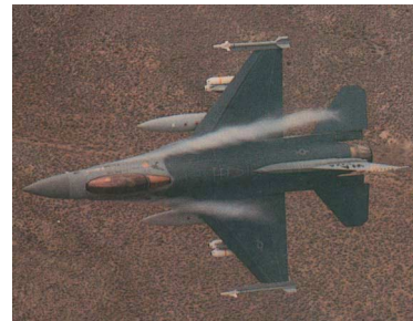
Fig 12 Asymmetric vortices on F-16 in sideslip
