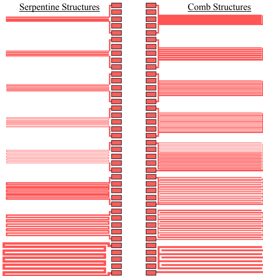
Figure 32. DISPLAYMETAL 1 Serpentine (left) and comb (right) test structures. This structure allows design rule validation and DISPLAYMETAL1 thickness monitoring.
