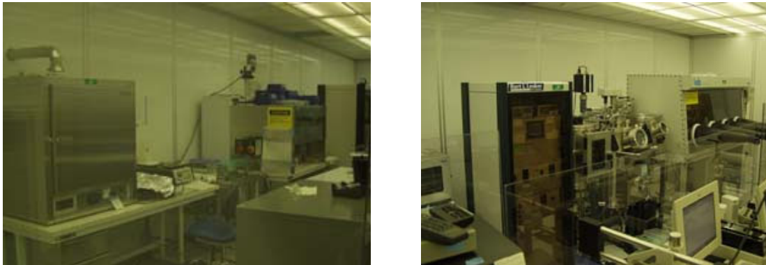
Figure 3. PLED Line after installation. Left: HPEA oven, spinner, and Class 10 flow hood. Right: Custom made evaporator and glove box.
