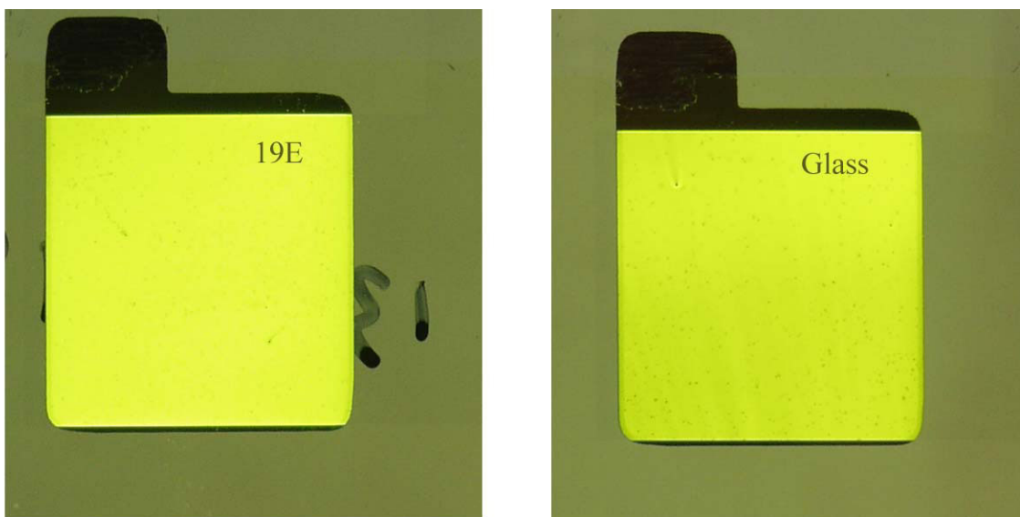
Figure 94. Fresh PLED devices encapsulated with Vitex 19E barrier (left) and with cover glass (right)..
