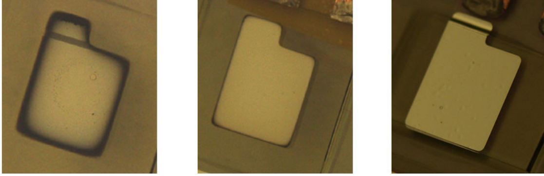
Figure 62. A view of the Ca/Al cathode of PLEDs fabricated on NB backplane with SU8 as the top layer. Left: substrate was baked in a vacuum oven for overnight before PLED processing Middle: substrate was baked for 10 days in the vacuum oven before PLED processing. Right: a 200nm SiO 2 barrier layer was deposited between SU8 and ITO.
