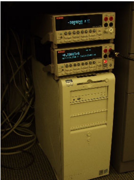
Figure 6. Semi automated I-V curve measurement setup consisting of Keithley power supply, computer and software (courtesy of Professor Yang Yang, UCLA)
