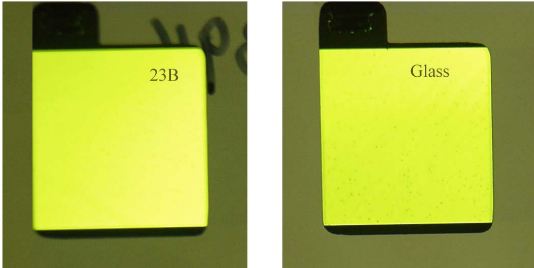
Figure 92. Fresh PLED devices encapsulated with Vitex 23B barrier (left) and with cover glass (right)
