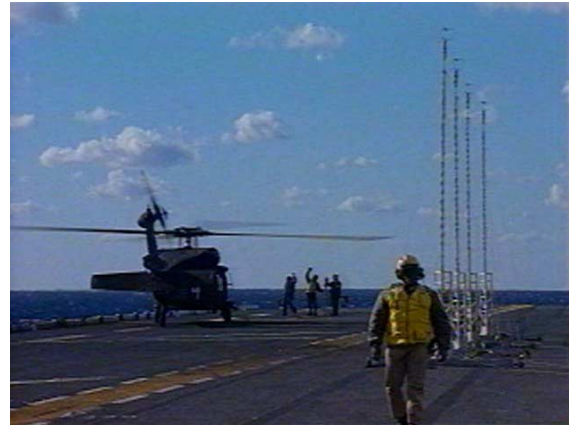
Fig 5. Four Ultrasonic Anemometers Atop 20ft Poles Used for Full-scale Data Collection
