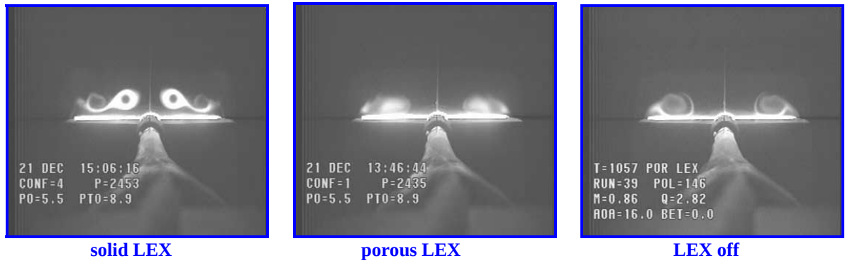
Fig. 6. Laser vapor screen images at Mach=0.85 and \alpha=16^\circ
