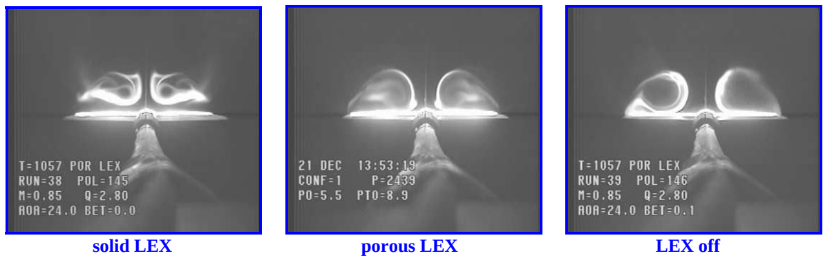
Fig. 8. Laser vapor screen images at Mach=0.85 and \alpha=24^\circ
