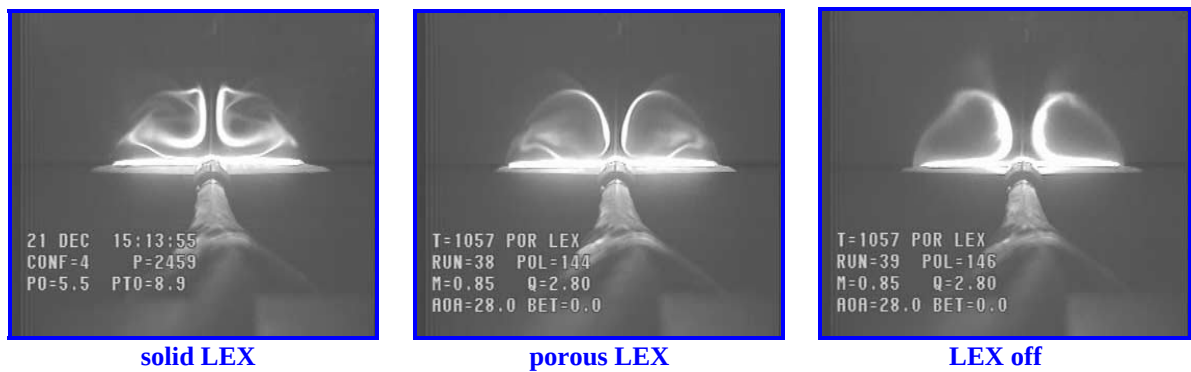
Fig. 9. Laser vapor screen images at Mach=0.85 and \alpha=28^\circ
