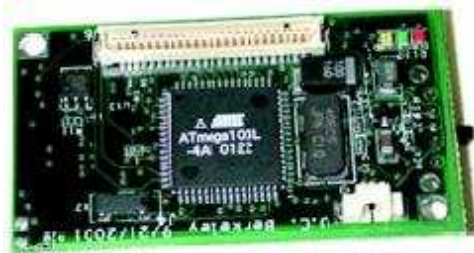
Figure 1: A Berkeley MICA Mote
