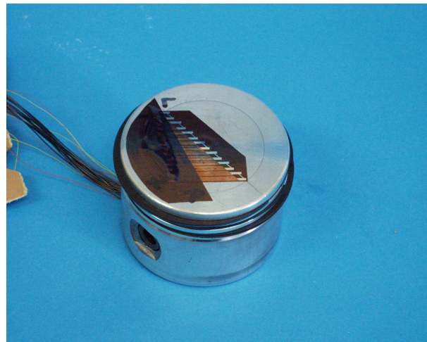
Figure 1b . Piston instrumented with thin films
