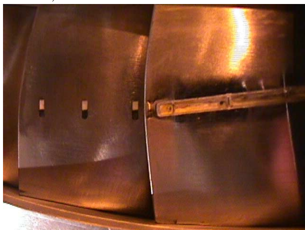
Figure 4 Vane Suction Side Pyrex Heat Flux Gauges and Pressure Transducers
