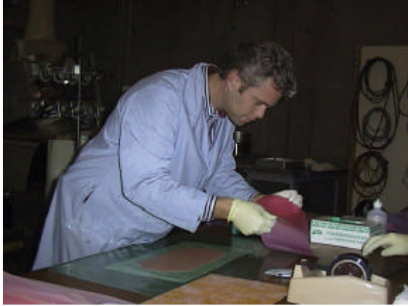
Figure 11.1-6. The patch was a) layed-up according to the designated configuration and b) carefully applied to the prepared surface.
