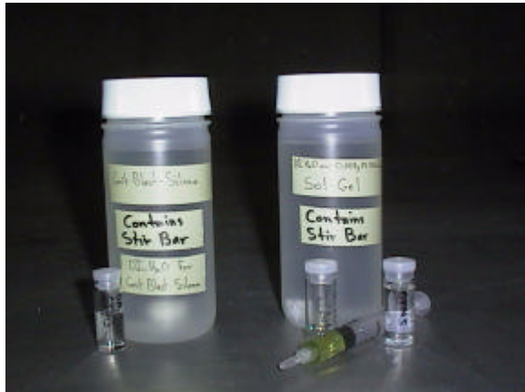
Figure 11.1-2. a) Grit-blast/silane and Boegel-EP11 kits ready for use; b) dirt, paint, and gross contamination is removed using Scotch-Brite® Roloc discs.
