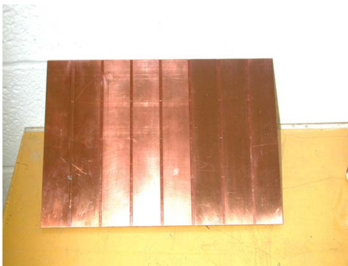
Figure 52: Thermocouple Mounting Plate
