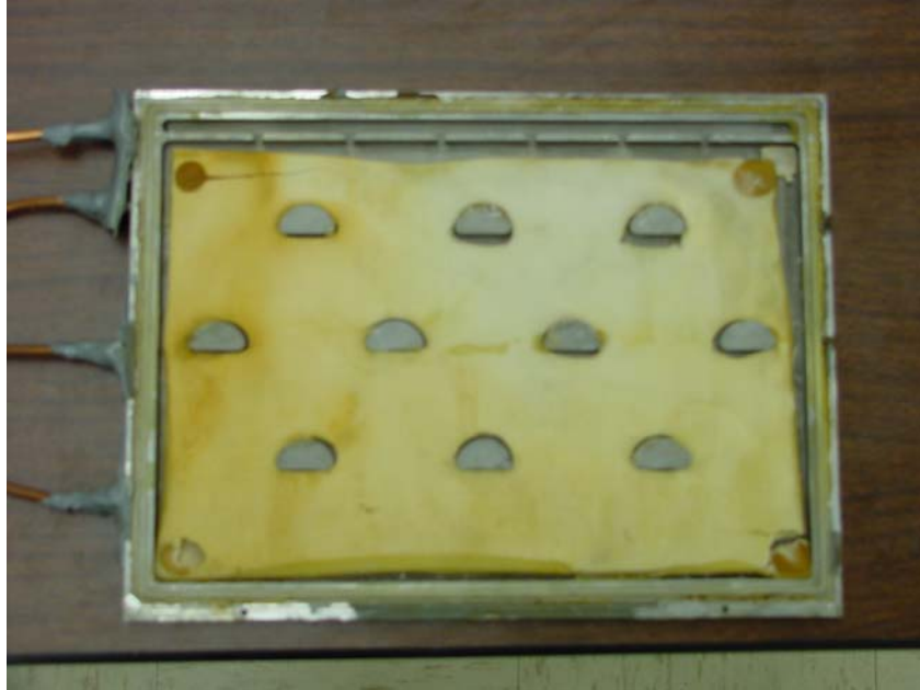
Figure 29: Aluminum Plate with Plastic Wick After Subcooling Tests
