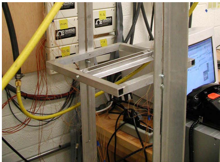
Figure 44: Tilt and Pitch Device. The device is located in the bottom half of the picture. This picture was taken before the evaporator plate was added.
