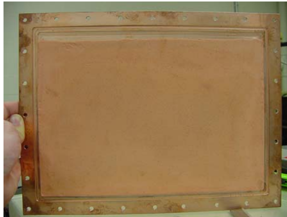
Figure 28: A 16.15 \mu\text{m} Sintered Copper Wick
