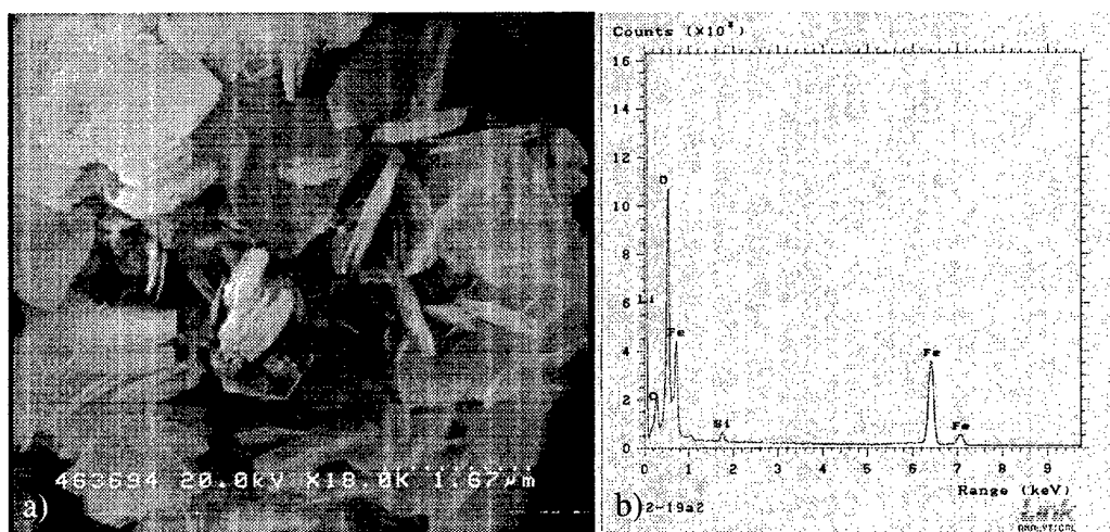
Figure 6.40. a) SEM image and b) EDX spectrum of Peerless iron, exposed to OU5 (OU12) TCE groundwater for 295 hours.
