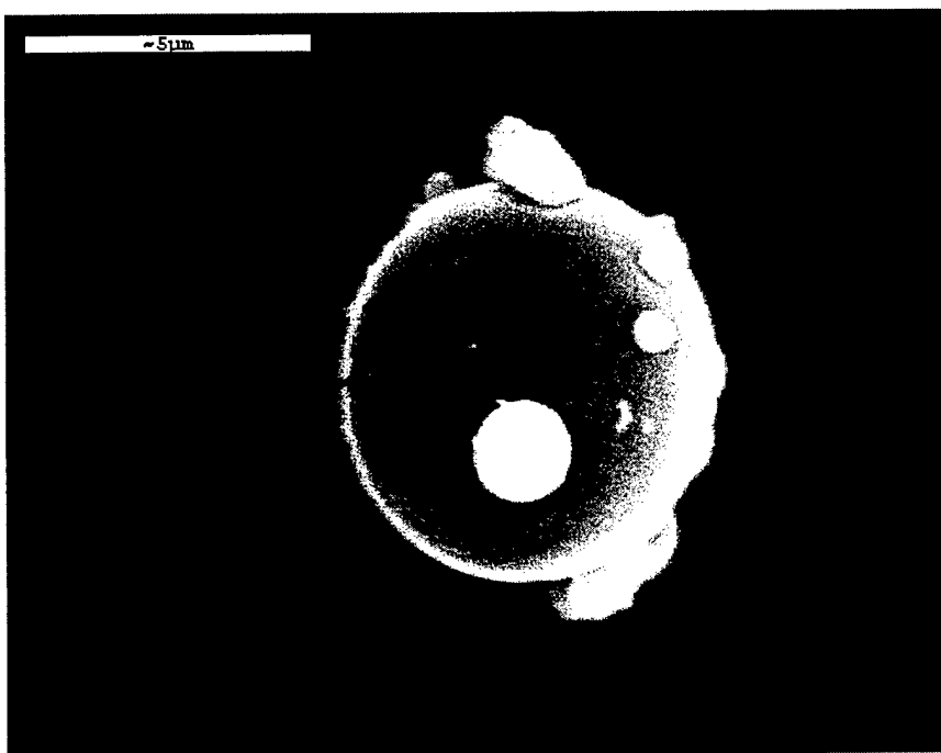
Figure 25. Undecenylamine grafted E-glass bead after 1 day exposure to TFAA.
