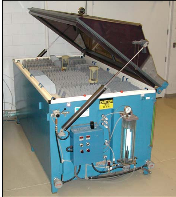
Figure 2. Test chamber and panels used for ASTM B 117.
