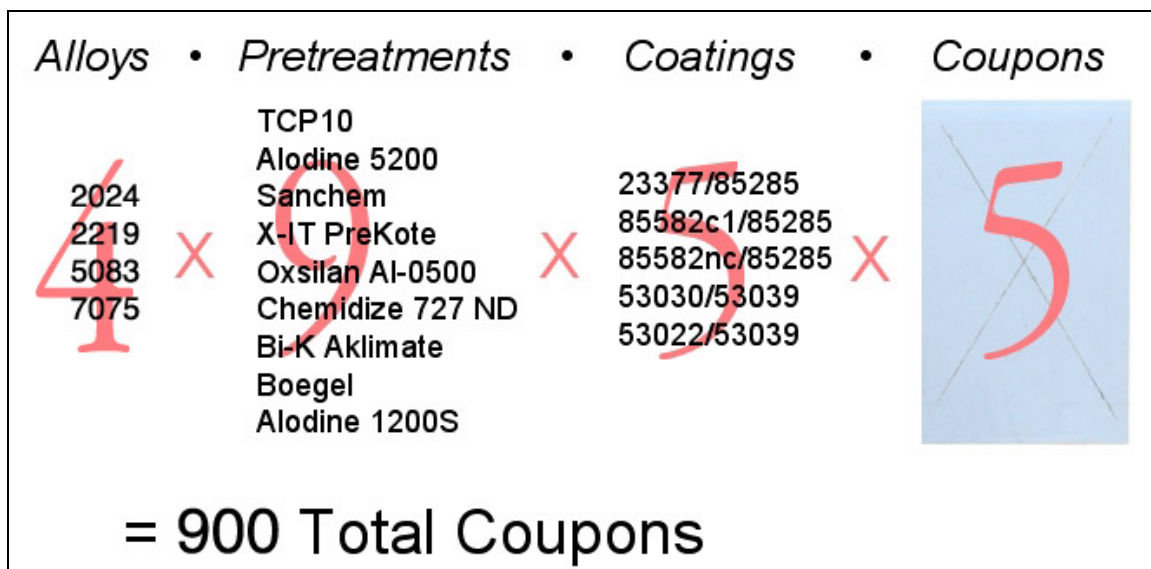
Figure 1. ASTM B 117 test panel matrix breakdown.
