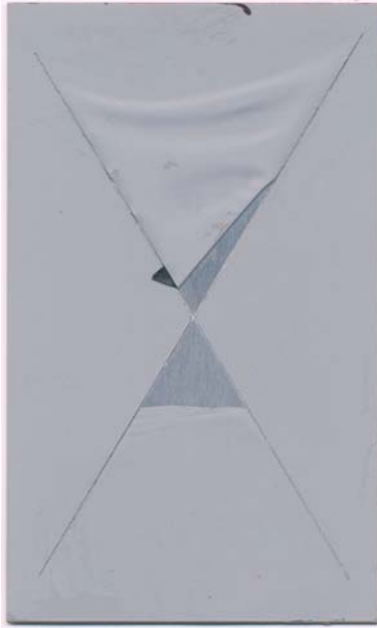
Figure 10. Severe delamination of Brent Oxsilan Al-0500 pretreated Al 7075 with 85582c1/85285 at 1 week ASTM B 117 exposure.
