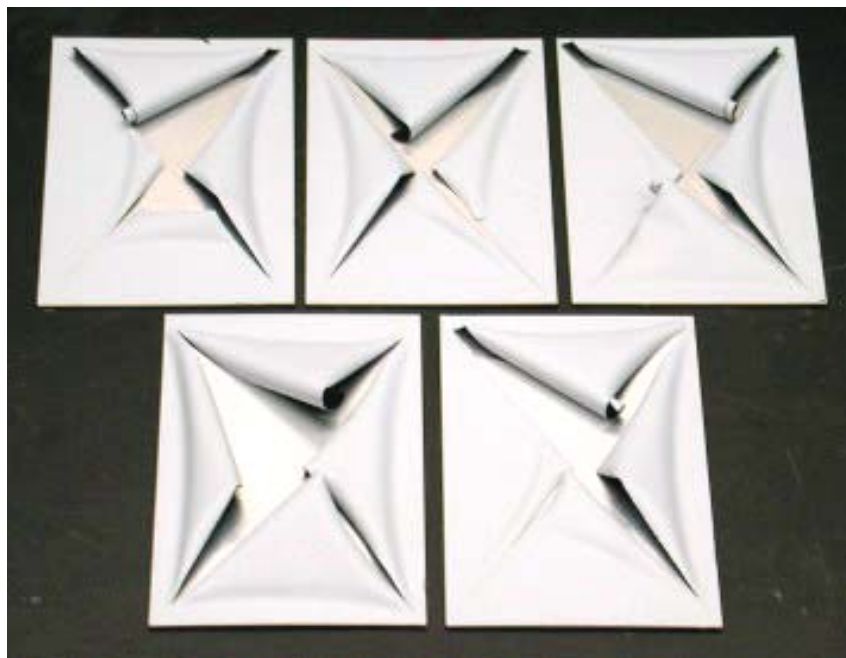
Figure 11. Severe delamination of Brent Oxsilan Al-0500 pretreated Al 7075 panels with 85582c1/85285 at 2 weeks ASTM B 117 exposure.
