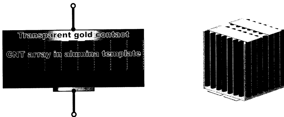
Figure 2. (left) One-pixel prototype of a CNT-based optical detector. (right) Addressable design using crossbar contacts to define detector pixels
