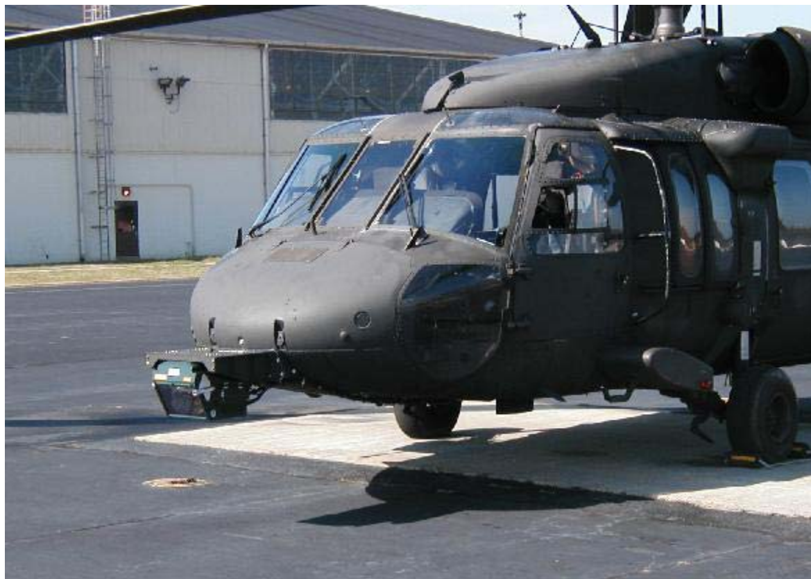
FIGURE 1: UH-60 BLACKHAWK WITH MOUNTED HELLAS OBSTACLE DETECTION SENSOR
