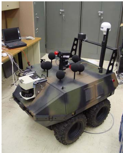
Figure 5. iRobot ATRV-2 robot with improved modular sensor platform.
