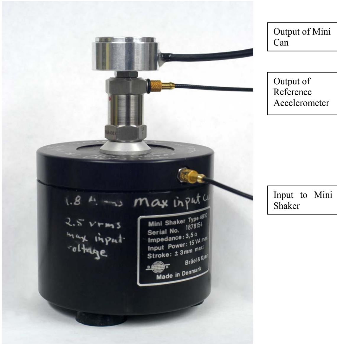
Figure 9. Photo of the arrangement used to obtain the Acceleration Sensitivity.
