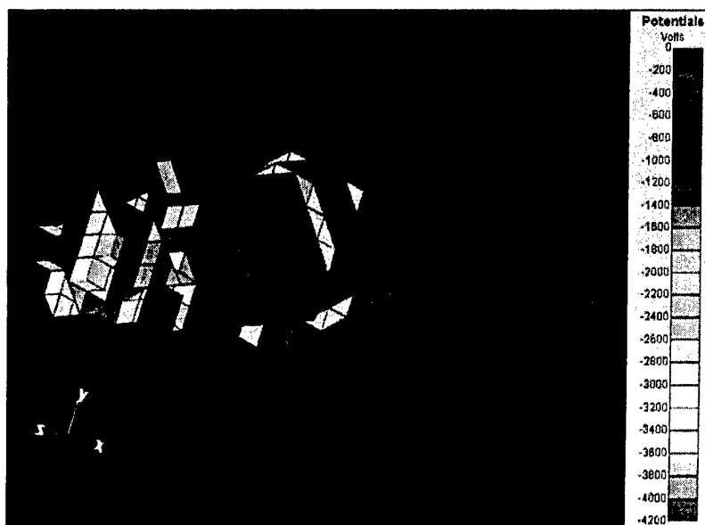
Figure 33. Resulting Surface Potentials for Case with All Teflon and Self-Consistent Charge Density.
