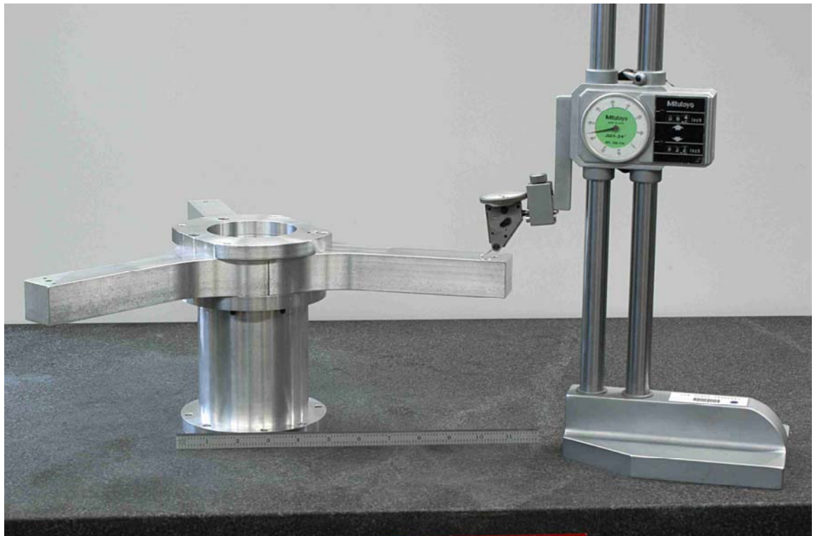
Figure 43. Central Cylinder, Top Optical Boomerang, and Verification Base Plate Substructure. Precision Height Meter and Precision Granite Table also Shown
