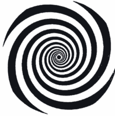
Figure 8. Four-arm logarithmic spiral antenna with self-complementary pattern (From Ref. [4].).
