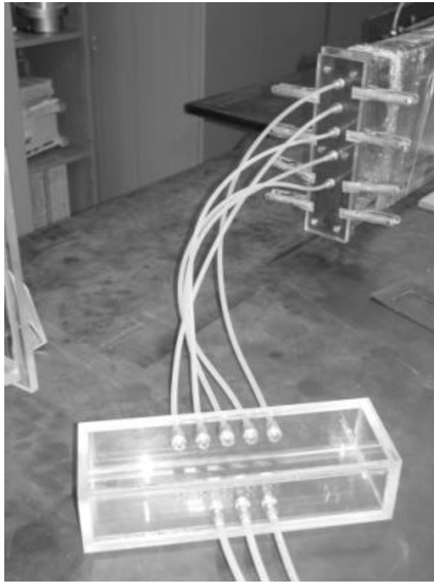
Figure 3. Air manifold section
