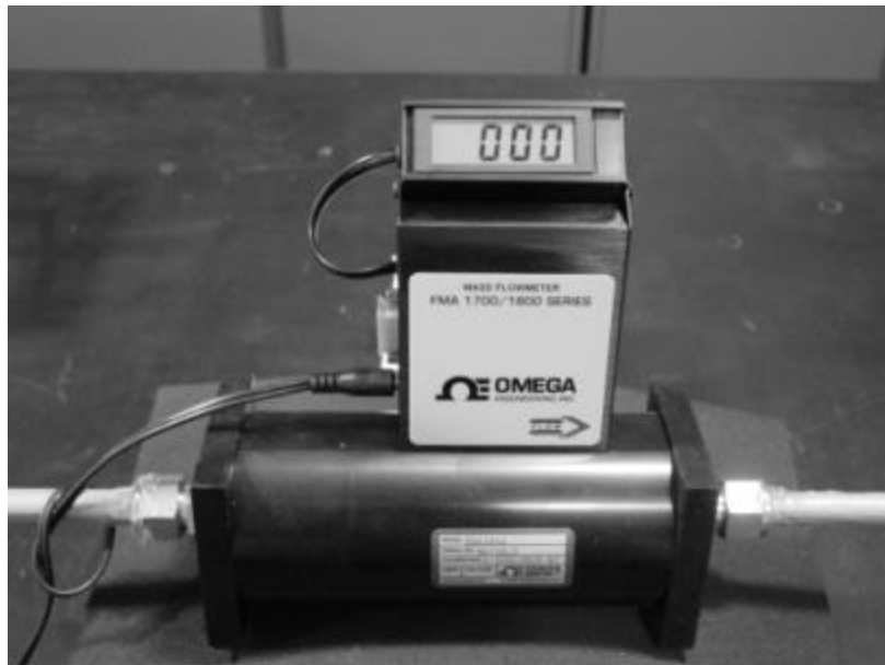
Figure 18. Omega FMA-1844 mass flow meter
