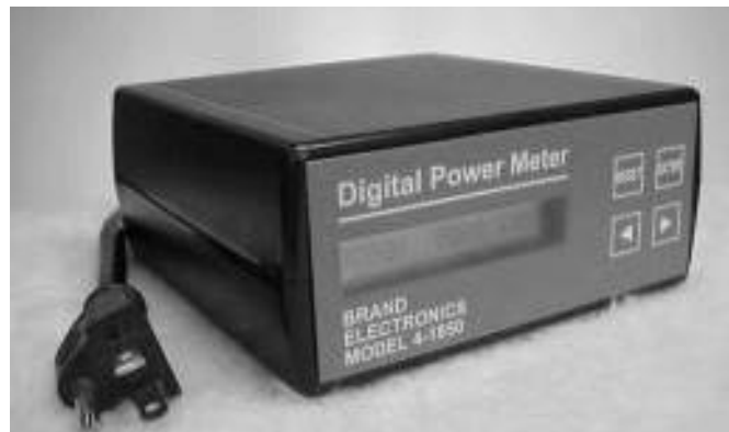
Figure 24. Digital power meter
